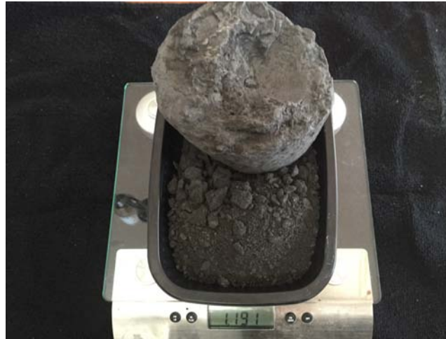
Image After Test 1.19Kg with Spall
